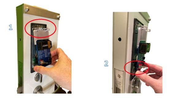
Remove tester by pulling the bottom out of the 60pin connector.
